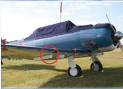
TYPICAL AOA PROBE LOCATION
