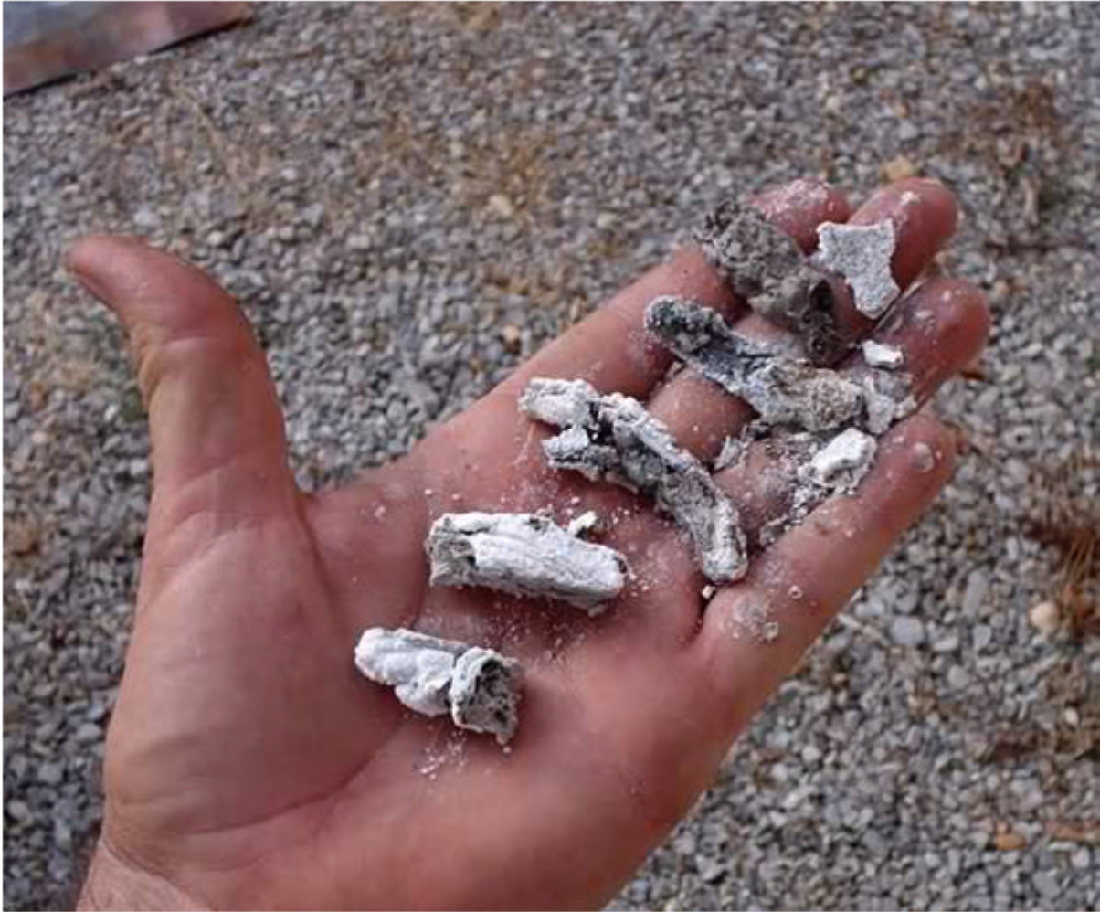
Note the CS1900 char still intact on the wire. It was tougher than the silicone chars. Also note the Resbond strips. Although entirely intact, they released from the stainless with no effort.
