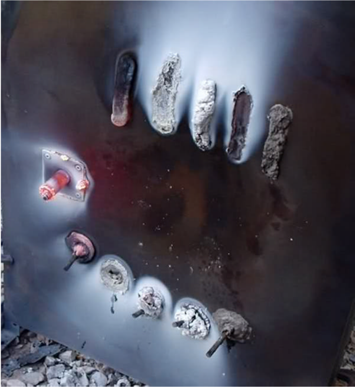
Hot-side chars collected post-burn. They are soft and fragile, puffballs really:
