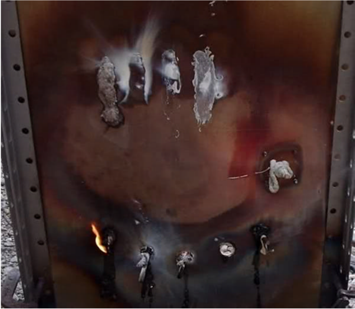
Front side again. The CS1900, FireBarrier, and Resbond strips are still hanging. The torch is aimed directly at the welded tube fitting, which is glowing red. In another minute or two the red hot copper wire core will ignite the tefzel insulation on the opposite side, at which point I ended the burn.
