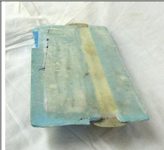
Picture 5 cover bonded to seat base
