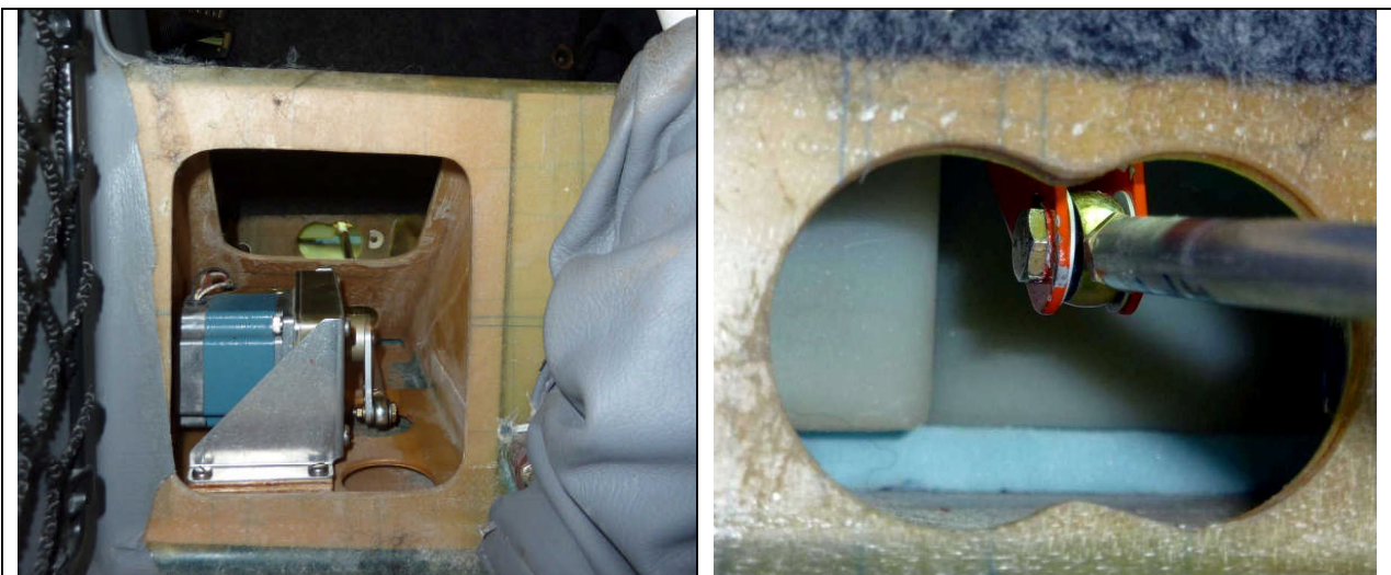
Picture 2 Example TruTrak installation.
