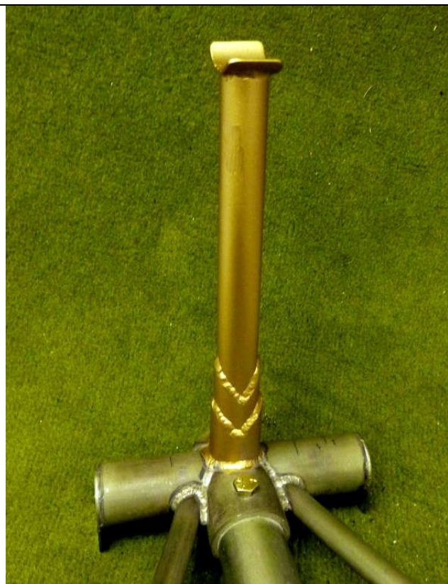
Picture 3 Reworked stop tube
