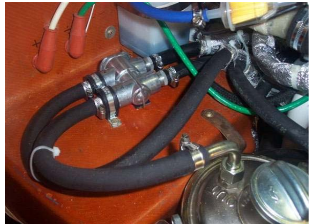
Figure 4 Example of valve installation in a Europa aircraft.
