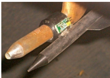
AOA Vane mounted next to Pitot tube.
