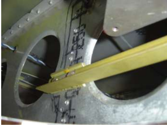
These three photos are my attempt to show the brace in place. This is on the left wing from front to rear in 3 exposures.
